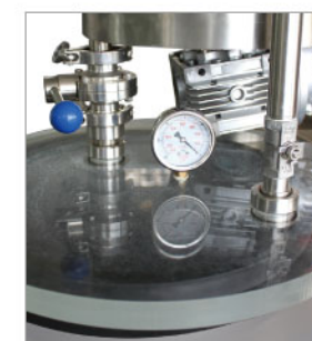
进口透明加厚亚克力板和全硅胶密封圈加大下桶 Imported transparent acrylic plate and thick silica gel sealing ring to increase barrel
