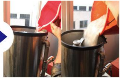
3、依次将水和石膏粉倒入不锈钢自动真空搅粉机上桶并盖上盖子。 3. Pour water and investment powder into the up chamber of automatic vacuum mixer and then cover on.
