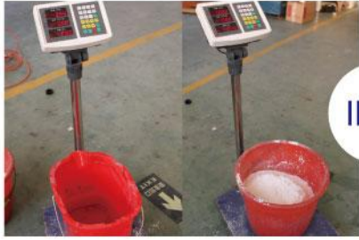
1、按比例称好所需的水和石膏粉。 1. Weigh water and investment powder according to the proportion.
