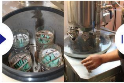
2、将装好蜡树的钢盅置入不锈钢自动真空搅粉机下桶并调整位置使其对准出粉口。 2. Put wax tree into flask, then put flask inside down chamber of vacuum mixer, then adjust the position of flask to make it right under the injection valve.
