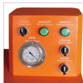
操控面板 Operation pannel
