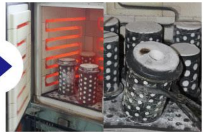
6、将烘干的钢盅放入不锈钢电炉内焙烧，待钢盅内的蜡充分燃烧蒸发后即可取出进行铸造。 6. Put the dried flask into stainless steel oven to heat, wait until wax is fully burned or evaporated, finally take out investment mold to start casting.
