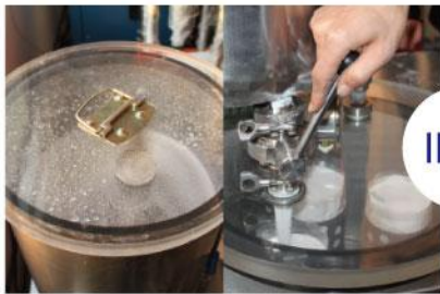
4、启动搅粉机开关进行搅粉，待搅粉均匀后拉出出粉口把手将搅好的石膏粉浆注入各个钢盅。 4. Starting mixing, after stirring the powder evenly, open the valve and inject mixed power into each flask.
